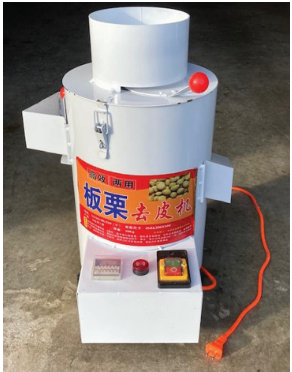
Figure 1. The mechanical chestnut peeler from China.
