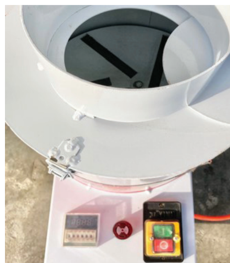
Figure 2. The peeling chamber on the unit.
