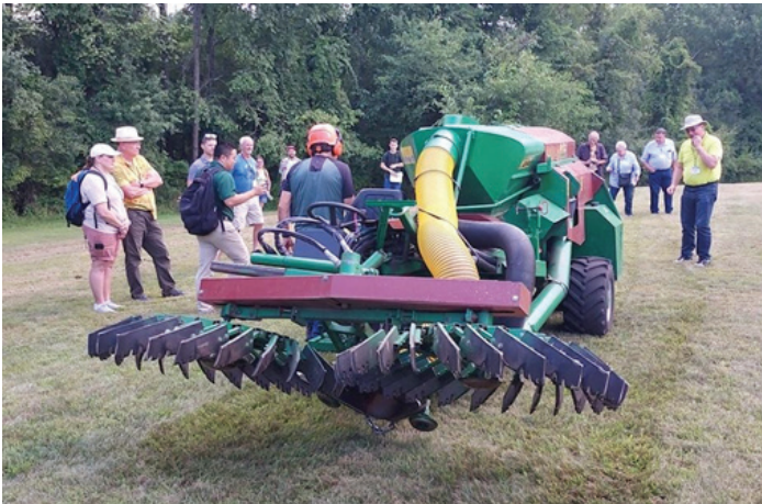
Fig. 3 – Dr. Mario Mandujano demonstrated use of a self-propelled chestnut harvester at Rogers Reserve.
