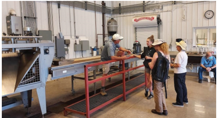
Fig. 4 – Part of the fresh chestnut peeling line at Rogers Reserve showing rack of rollers to remove charred pellicles and table for visual inspection of peeled fresh chestnuts.
