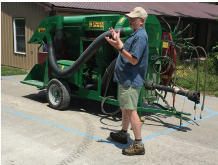
Mike Gold explains: The FACMA harvester sweeps burs into a row, vacuums them up, separates the nuts from the burs, and then throws the debris back under the trees. To use it effectively, the ground needs to be near perfect – mowed, flat, and clean.
