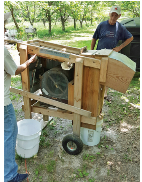
Examining a dry cleaning machine fabricated by Charlie that saves a tremendous amount of time during the cleaning phase of the nuts.
