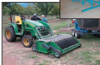
Left: Harvesting with a front-loader adapted with “fingers” for picking up chestnuts and burs. The fingers pick up the burs and nuts and drop them
