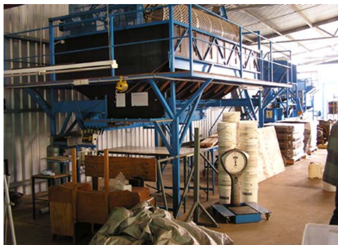
There are advantages to using dual sorters. It allows the Renaudos to process about 2000 pounds an hour. With a large orchard and the cost of labor that's seen as very important.
