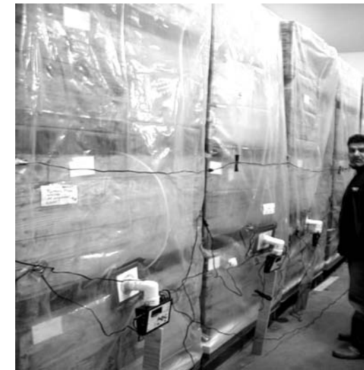
Figure 4: Several CALM Units running showing the bins of chestnuts in plastic tube and sealed to pallet base.
