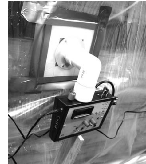
Figure 3: Current CALM Model V6 sealed to chestnuts in plastic tube with interface plate.
