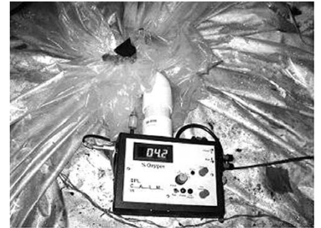
Figure 2: The second model involved moving the sensor well away from the heat of the electronics and placing it within the plastic bag.
