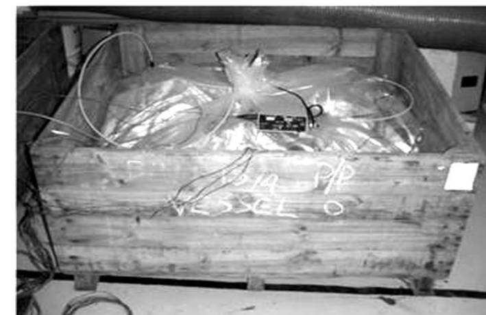
Figure 1: The first model involved the controller being stuck onto the plastic bag enclosing the nuts, the body of the oxygen sensor being in the controller box and the large plastic bag sealed by twisting the bag and using a cable tie.
