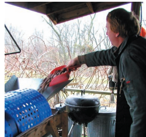
Tom Wahl loads a batch of fresh chestnuts into the size sorter. The first bin has holes for tiny chestnuts to fall through, the next has small-sized holes, then large and extra large.
