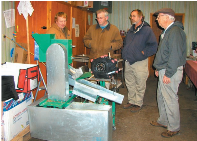
Bottom: Winfield Tree-grown Foods uses a modified peanut sheller to peel chestnuts. Left: Tom Wahl, (far left) Mike Gold, Ken Hunt and John Wittrig discuss the peeling process. Top: The nuts move through a cylindrical screen, and then rotating bars crush the shells. The kernel falls through the screen and a blast of air removes any shell fragments.
