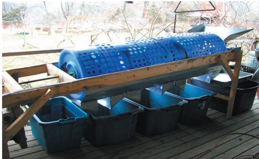
Chestnuts are poured into the chute (right), then a set of motors turns the plastic drums. Nuts fall through the appropriate sized holes into bins below. When nuts are no longer falling into the bin below, the machine operator flips a reverse switch and the nuts shift into the next size drum until all the chestnuts have been sorted by size: tiny, small, large or extra large.
