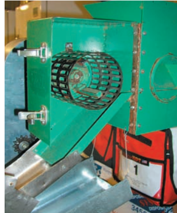
Bottom: Winfield Tree-grown Foods uses a modified peanut sheller to peel chestnuts. Left: Tom Wahl, (far left) Mike Gold, Ken Hunt and John Wittrig discuss the peeling process. Top: The nuts move through a cylindrical screen, and then rotating bars crush the shells. The kernel falls through the screen and a blast of air removes any shell fragments.
