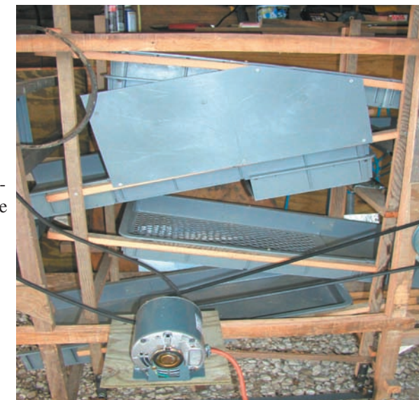
Once peeled, chestnut kernels (top) are sized and cleaned by this machine. Each tray has holes drilled in the bottom, and as the shelled kernels slide down the trays, various size holes allow kernel pieces to fall through while a fan blows the debris or shell fragments away.
