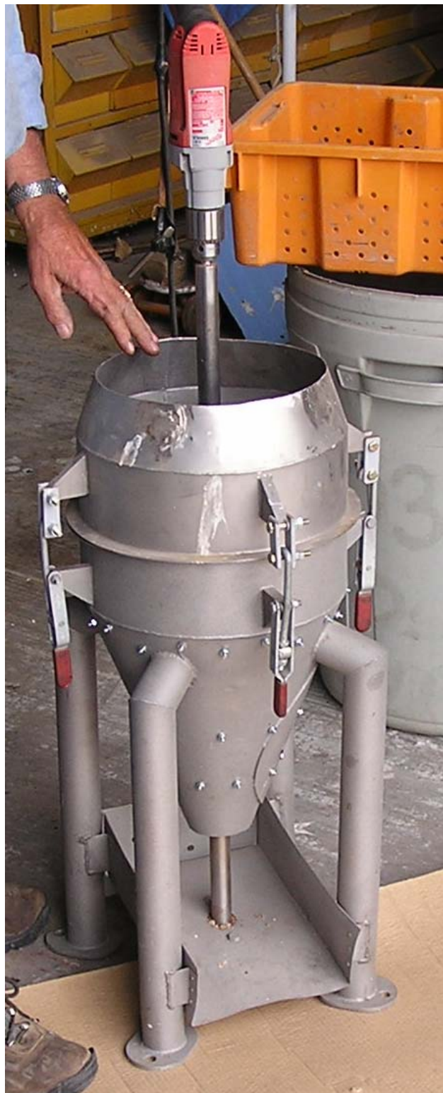
This machine is used to scarify the nuts prior to being peeled. It's lined with wood rasps on two surfaces.
