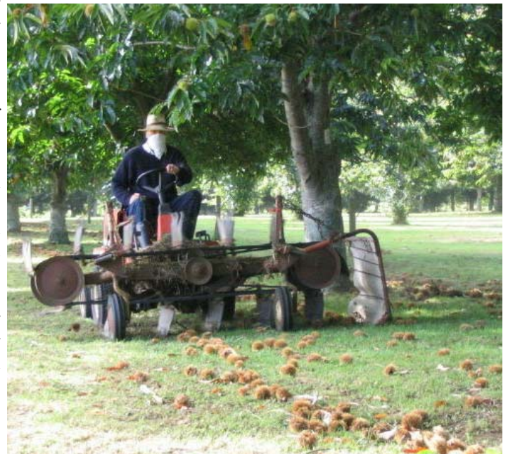
Nick Empson, wearing dust mask, operating his sweeper derived from a Kubota mower and a hay sweeper.
