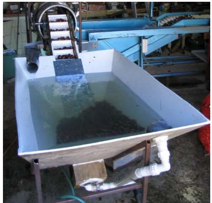
Hugh Beecroft's initial washing apparatus, an inverted pyramidal tub for floating off culls with conveyor into a 2 nd stage washing, a tumbler cylinder.
