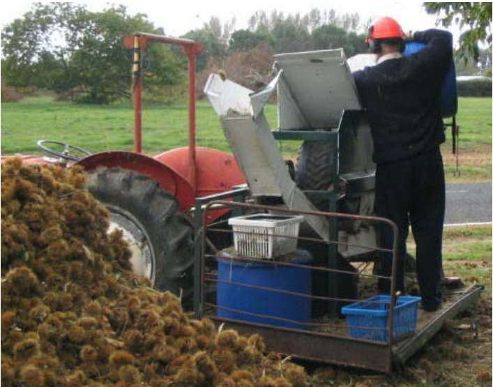
Nick Empson, with helmet and hearing protectors, operating his home-built deburring/cleaning machine.
