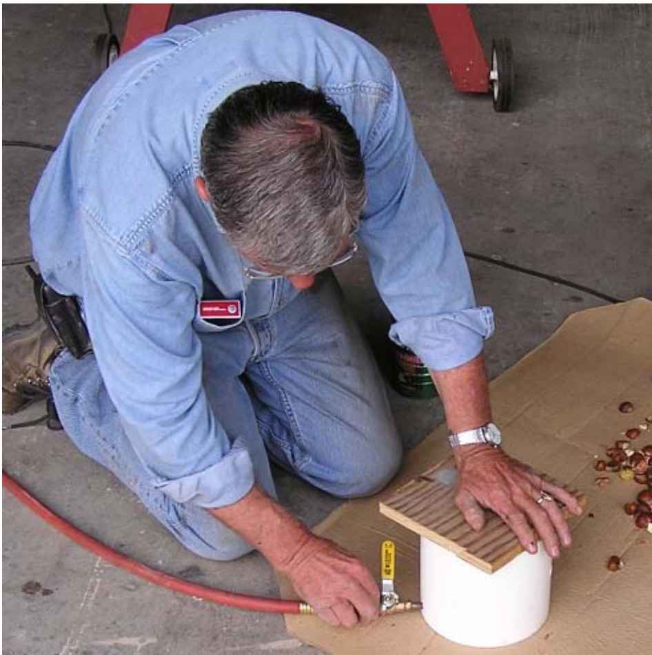
A blast of air causes the scarified nuts to bounce off the wood rasps that line the inner surface of the tube.
