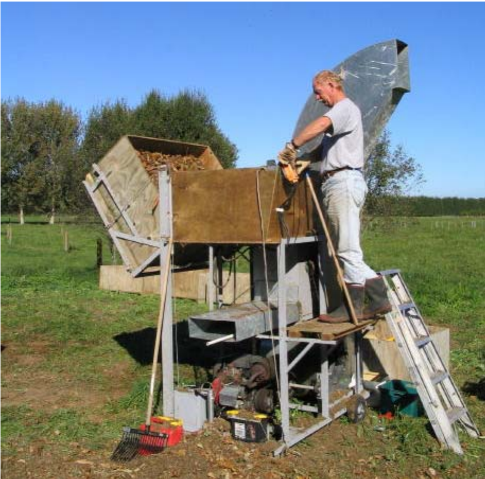
Hugh Beecroft demonstrates the machine he built. This machine, with its duct tape deburring cylinders, processes burrs and all orchard sweepings, separating the chestnuts in an air tunnel from the refuse with 90% efficiency, he estimates.
