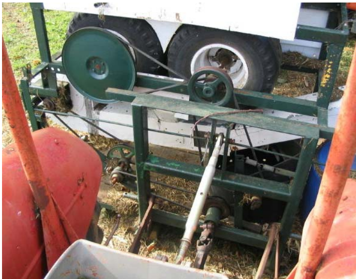
Nick Empson deburrer/cleaner, showing the drive-train attachments to tractor PTO and the belt system used to drive the counter-rotating tires and the fan.
