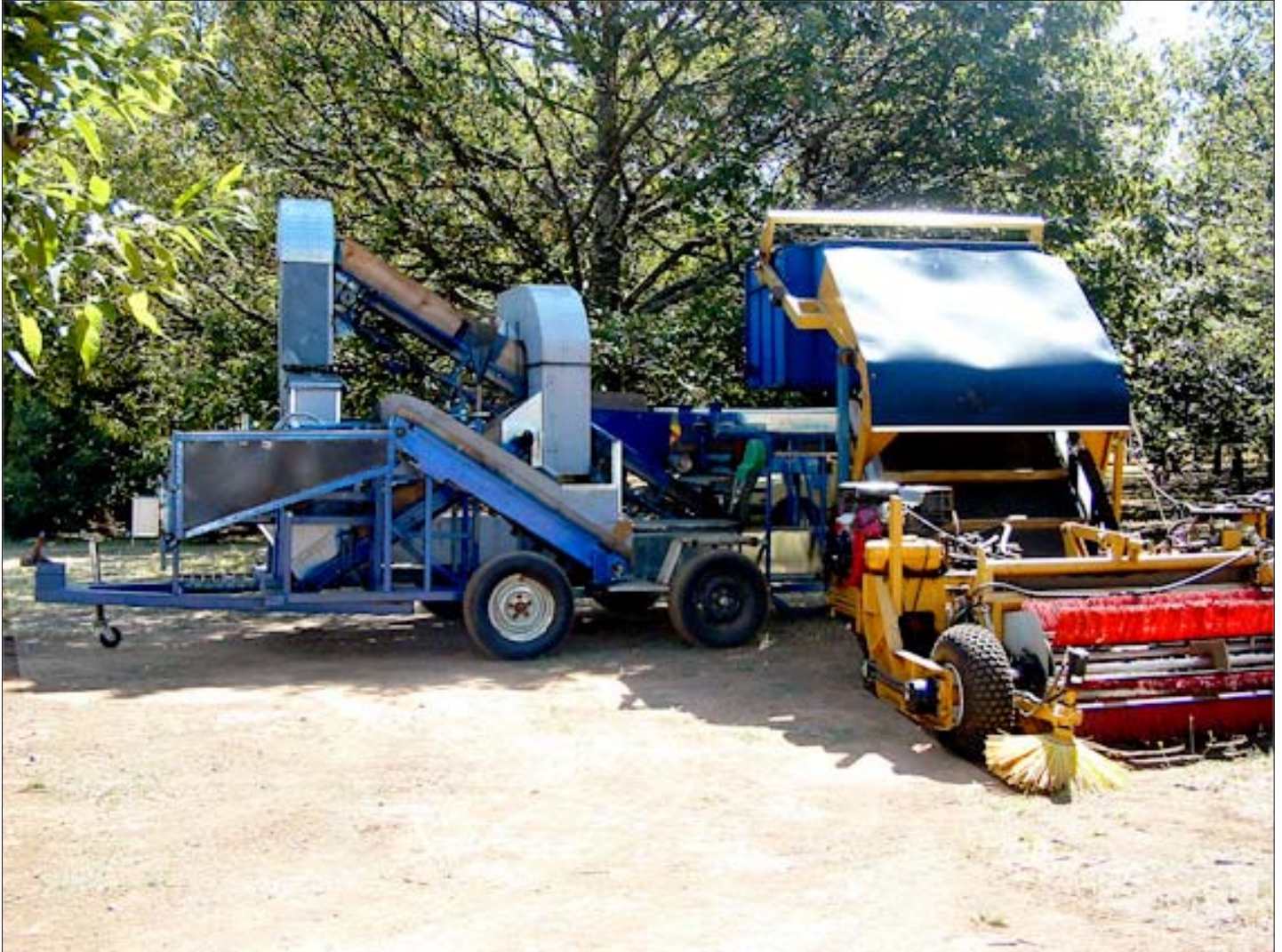
The Turnbull Multi-Nut harvester unloading into the mobile De-Burrer. (Photo: George Turnbull.)
