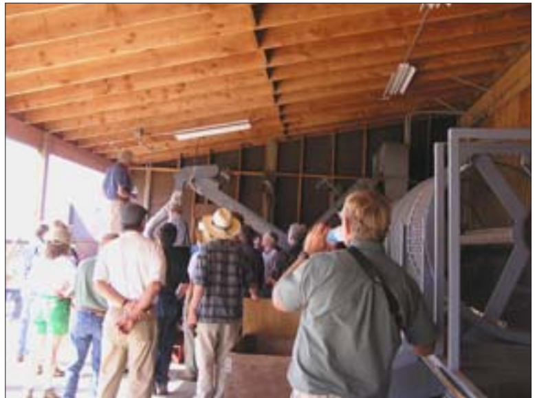
Ben Bole explains his custom designed processing line at Ladd Hill Orchards. Nuts are fed into a hopper and proceed to an air leg where the hulls are separated. Nuts proceed to the sorter at right.
