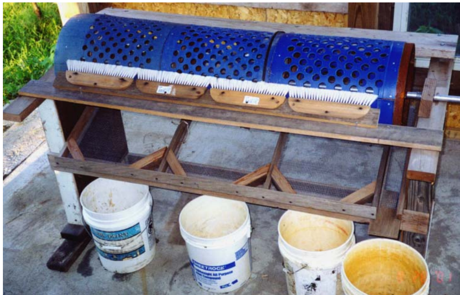
The finished sorter is shown complete juice barrels, wallpaper brushes to keep the nuts moving, hardware cloth and other easily obtained materials. Cost to build was about $100.
