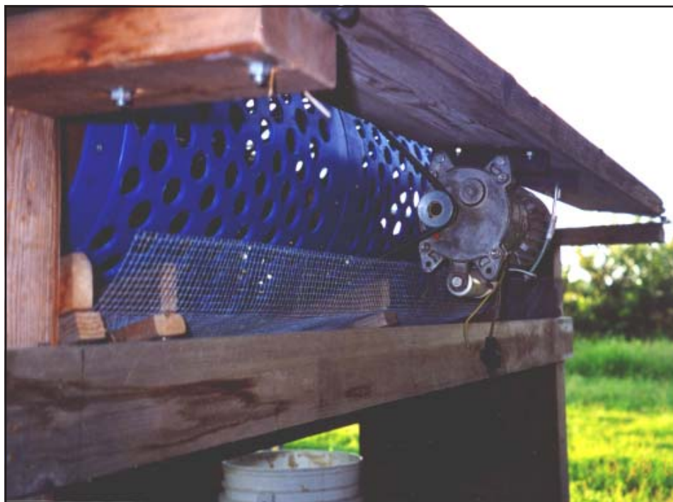
The view from beneath the sorter reveals the scrap gear-reduction electric motor which drives the unit using an automotive fan belt surrounding the barrels.
