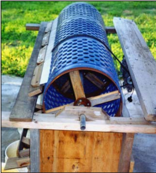
An end view of the sorter reveals the 1"x2" wooden spokes mounted on a 3" sheet metal rim. The axle is electrical conduit.
